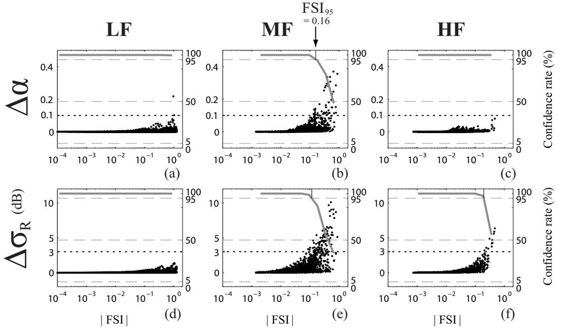
FIG. 6. Evolution of the difference between the Biot and limp models as a function of  $FSI$  for the two configurations including the 256 simulated materials of thickness 2 cm: (a)-(c) absorption coefficient, (d)-(f) radiation efficiency of a covered plate; in the three frequency ranges: (first column) Low frequency band **LF**, (second column) Medium frequency band **MF**, (third column) High frequency band **HF**.
