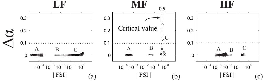
FIG. 5. Difference between the Biot and limp models on the absorption coefficient  $\alpha$  of 2 cm thick materials A (\*), B (•) and C ( $\times$ ), functions of their  $FSI$  parameter in the three frequency domains: (a) low frequency band, (b) medium frequency band, (c) high frequency band.
