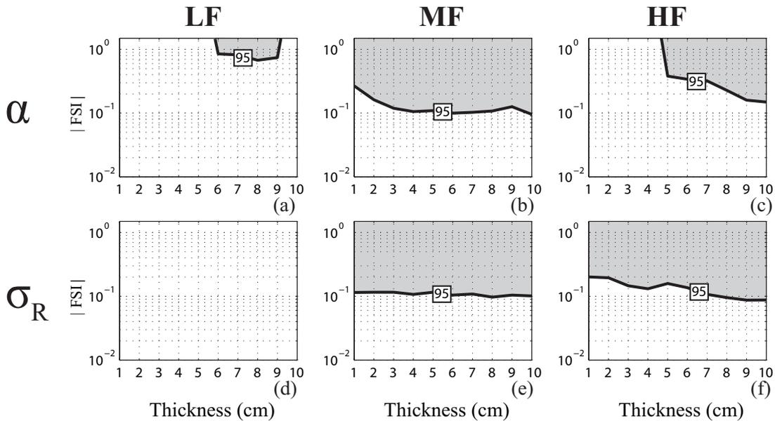
FIG. 8. Evolution of the  $FSI$  critical values as function of the thickness for the two configurations ((a,b,c): absorption coefficient, (d,e,f): radiation efficiency) in the three frequency ranges: (a,d): Low frequency band **LF**, (b,e): Medium frequency band **MF**, (c,f): High frequency band **HF**. White zone: limp model valid, Grayed zone: limp model not valid.
