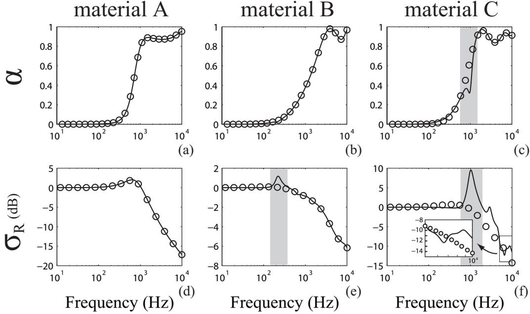
FIG. 4. Vibroacoustic response of the two configurations including the three real materials A, B and C of thickness 2 cm: (first line) absorption coefficient  $\alpha$ , (second line) radiation efficiency  $\sigma_R$ : (—) Biot model, (○) limp model.
