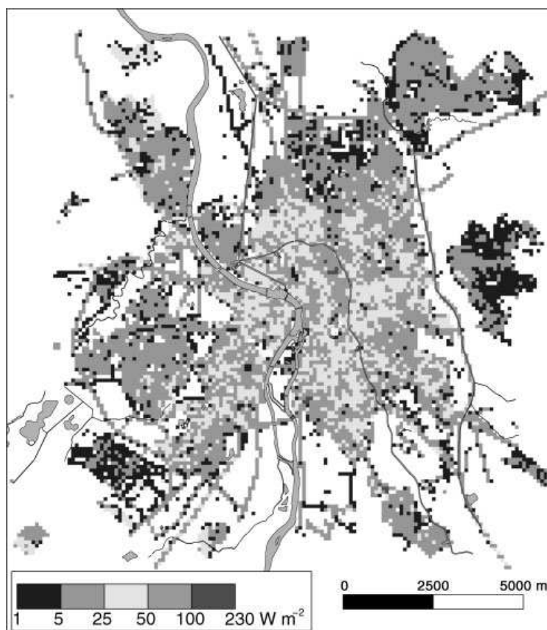
Figure 10. Spatial variation of Q_F over the agglomeration, averaged over December 2004, January and February 2005. This figure is available in colour online at www.interscience.wiley.com/ijoc
