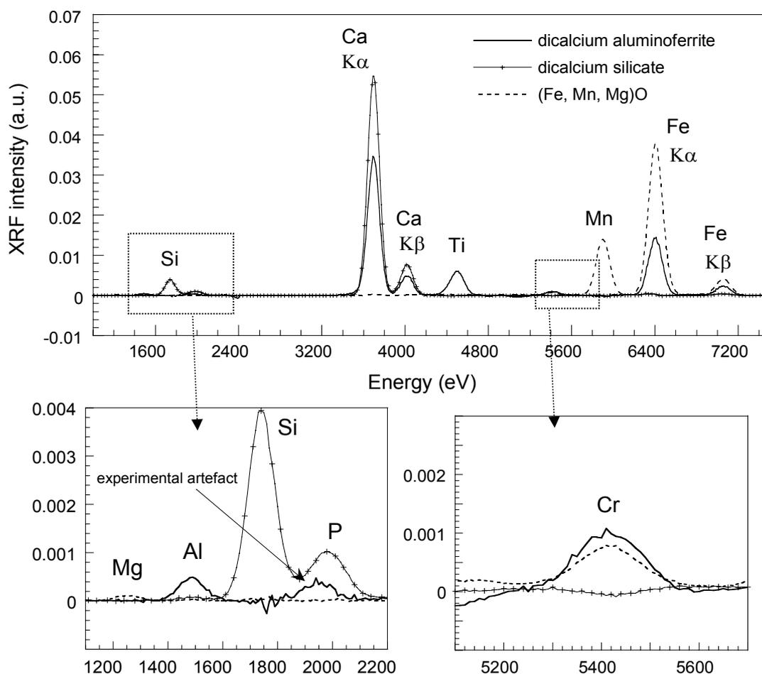
Figure 2. Resolved spectra obtained with the SIMPLISMA procedure (analysis of Lab-MXRF spectra of unaltered BOF slag, see ACP plot) from Ti, Si and Mn as “pure variables”
