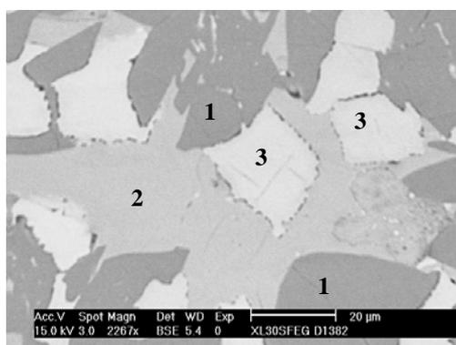
Figure 1. SEM photography of a BOF slag polished section (grains > 2 mm)
