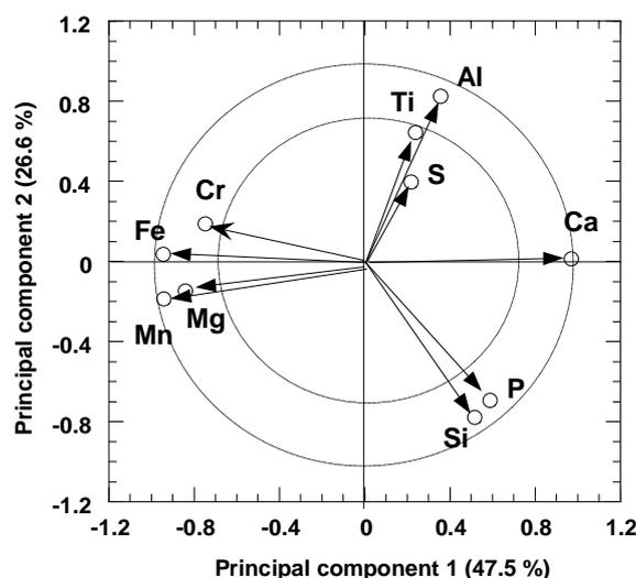
Figure 1. Principal Component Analysis (PCA) loading plot obtained from Lab-MXRF spectra (143 spectra of unaltered BOF slag, 10  $\mu\text{m}$  spot size, 15 kV, counting time of 1000 s) with a so-called “R” software (19). Variables, i.e. XRF  $K_{\alpha}$  lines intensity of each element, are plotted.
