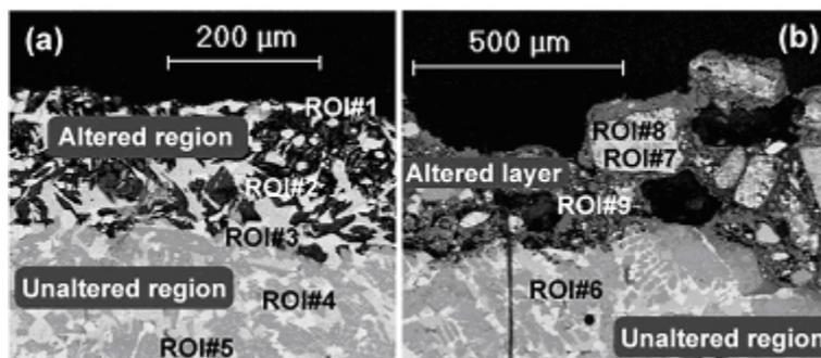
Figure 6. SEM-BSE micrographs of polished steel slag grains embedded in epoxy resin and previously leached at a laboratory scale (a) and in lysimeter (b). Regions of Interest (ROI) selected to record micro-XANES spectra with the focused X-ray beam are indicated (ROI#1 to ROI#9). ROI#4 to 6 are in the unaltered region, ROI#1, 2 and 9 are in the altered region and ROI#3, 7 and 8 are in little altered regions.
