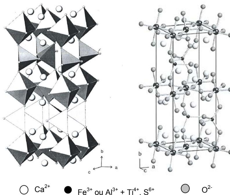
Figure IV-14 : Structure de la Brownmillerite  $\text{Ca}_2\text{Fe}_{2-x}\text{Al}_x\text{O}_5$
