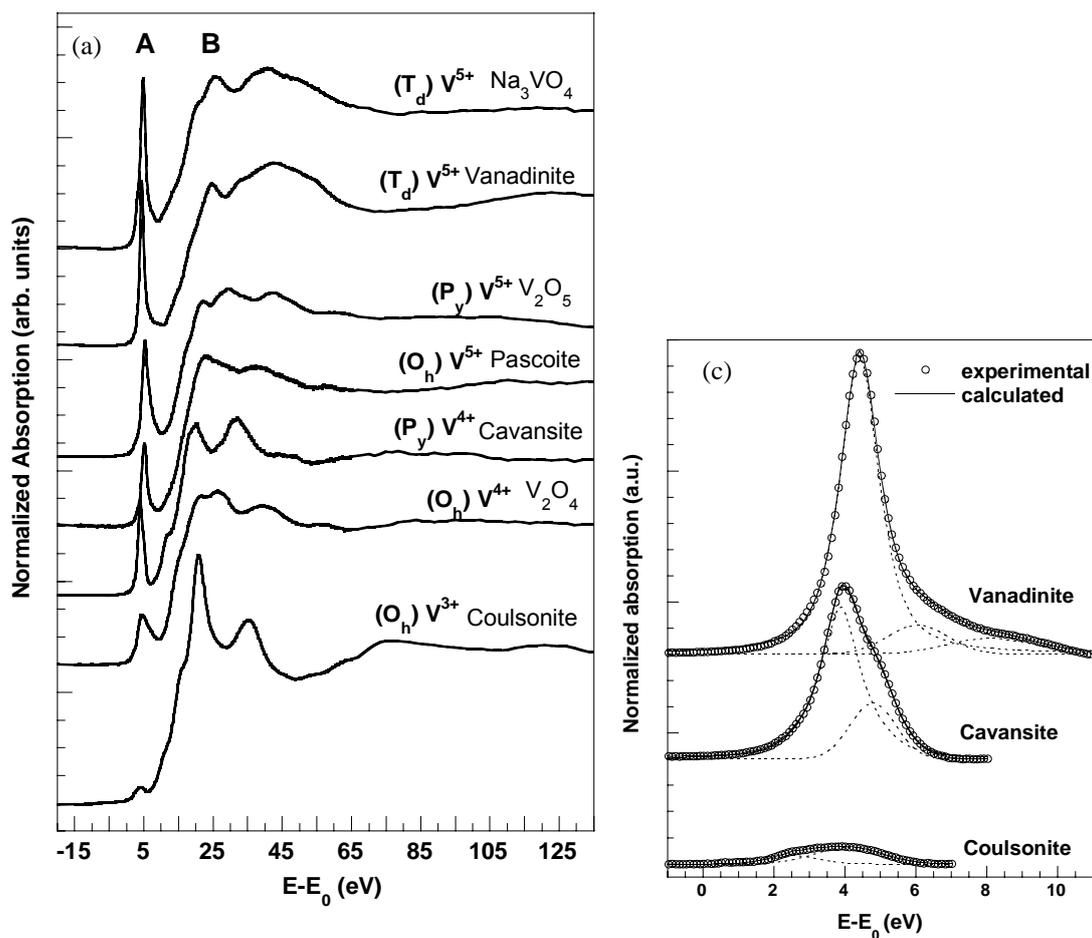
Figure 1. (a) Experimental V K-edge XANES spectra of standard compounds with V in different oxidation state (i) and symmetry (s): (s) $V^{i+}$  (recorded on beamline FAME, CRG-ESRF). (b) The pre-edge background was modeled with an interpolation function (baseline) using data a few eV before and after the pre-edge. (c) Selected normalized pre-edge peak of standard compounds and the best model calculated with 1 to 3 contributions.
