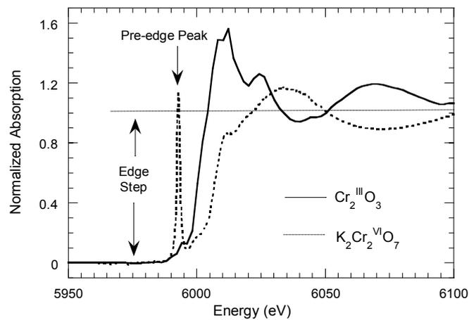
Figure 3. Normalized K-Cr XANES spectra for Cr standards:  $K_2Cr_2^{VI}O_7$  and  $Cr^{III}_2O_3$
