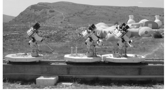
Fig. 1. The GSM configuration at Calern Observatory near the GI2T interferometer. Only four of the six GSM modules are presented here.
