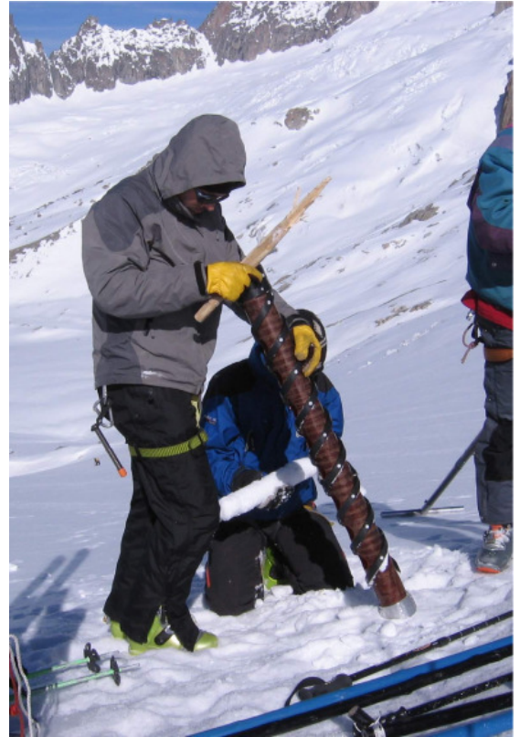
(c) Carottage de surface au printemps en zone d'accumulation. Shallow cores in spring in the accumulation zone.
