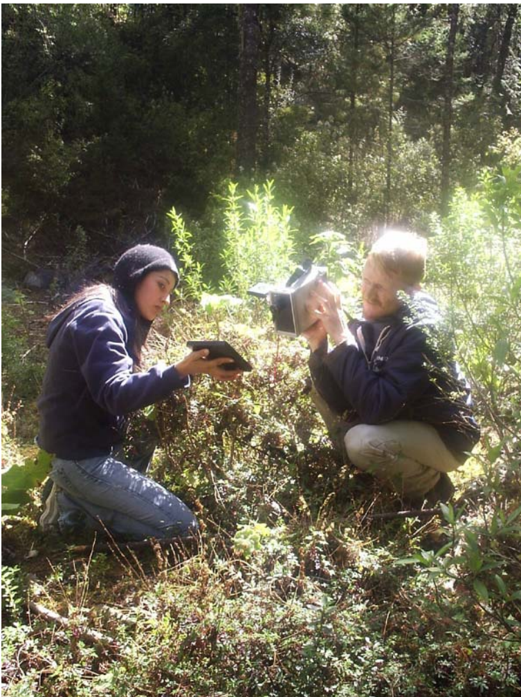
Photograph B.6: Radiometric measurement of fir ( Abies Religiosa ) forest understory. Isela Zermeño.
