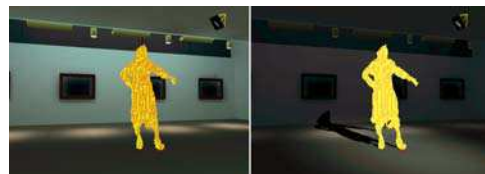
Figure 15: Marching cube representation: Shadow due to a virtual light. Left: the actor seems to be "flying" above the floor. Right: shadows remove this impression
