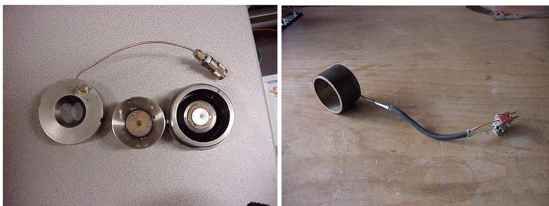
Figure 3.7: *Chervin-type DAC (left panel) and external heater for Chervin-type cell (right panel).*
