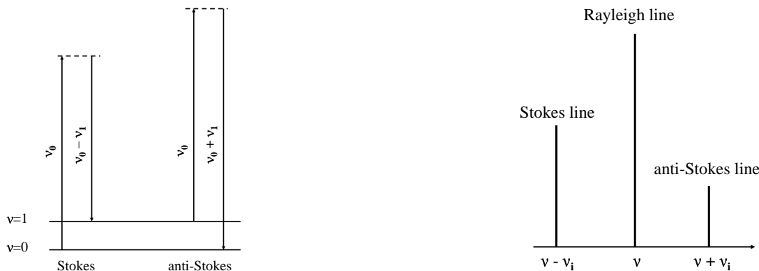
Figure 2.3: Mechanism of Raman scattering (left panel) and schematic view of a Raman spectra (right panel). The Stokes and anti-Stokes lines are symmetric compared to the Rayleigh line (elastic scattering). The intensity of the Stokes lines is always higher than the anti-Stokes lines due to the Maxwell-Boltzmann distribution law.
