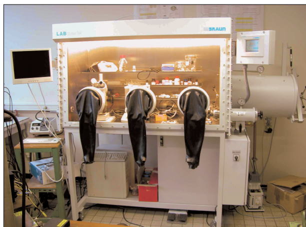
Figure 8.11: Picture of the glove box employed during the sample synthesis in order to avoid reaction or contamination of both the Rb and Cs alkali metals and the final Rb_6C_{60} and Cs_6C_{60} compounds.
