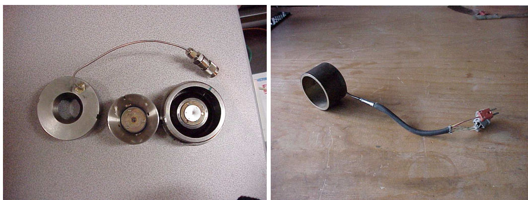
Figure 3.7: Chervin-type DAC (left panel) and external heater for Chervin-type cell (right panel).
