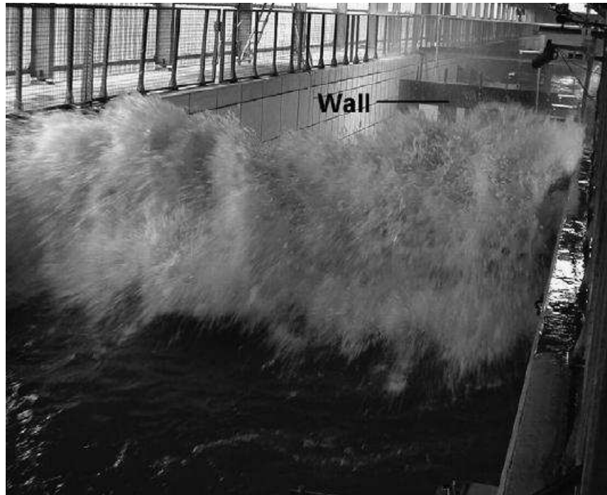
Figure 3.1: Example of homogeneous water/air mixture just after the wave breaking. This image is taken from [BOPB07].
