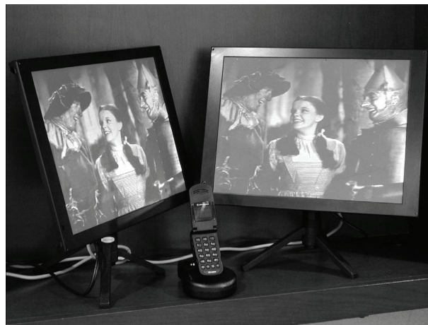
Figure 2–18 : Ecrans de type Field Emission Display de Motorola
