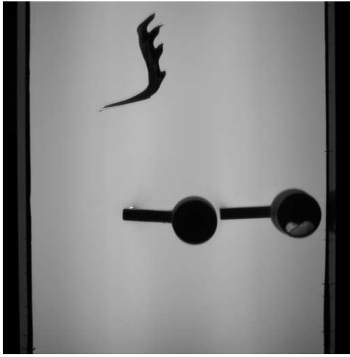
Figure 3.13: A dye blob initialized with no intersection with \mathcal{W}_s has been carried away downstream without being caught by the rods. Mixing is very inefficient for this initial condition.
