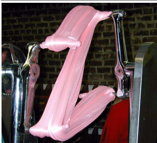
Figure 3.8: Four-pronged taffy puller. In this candy machine, the four rods braid in a non-trivial way and hence stretch taffy exponentially. As taffy is pulled tight on the rods – contrary to material lines in fluid flows –, the interface growth rate is exactly the topological entropy of the rods braid.
