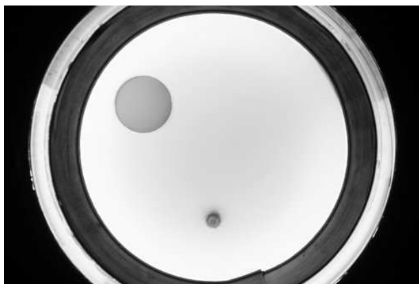
Figure 2.7: Example of picture used to calibrate the camera. A small transparent dish filled with a 1 mm-thick dye layer of known concentration value floats on the fluid surface. The layer thickness was chosen to approximate the thickness of the initial dye blob in experiments (Fig. 2.6).
