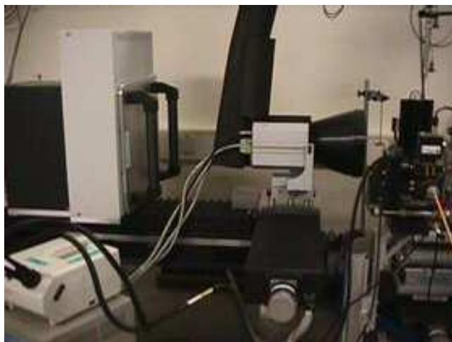
Figure 4.7: Photograph of the image plate detector, MAR345, used at the ID30 beamline.
