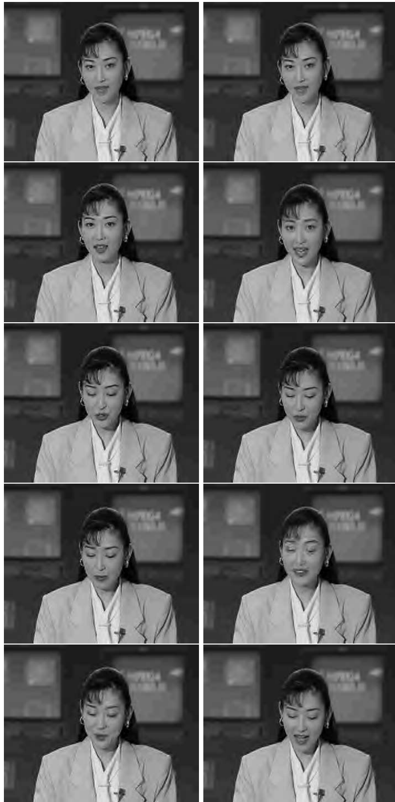
Figure 4.15: CIF akyio video compressed to 300 kbits/s (30 frames/s). Transmission over Gaussian channel at 0.001 ber. Using the SDC+TC.
