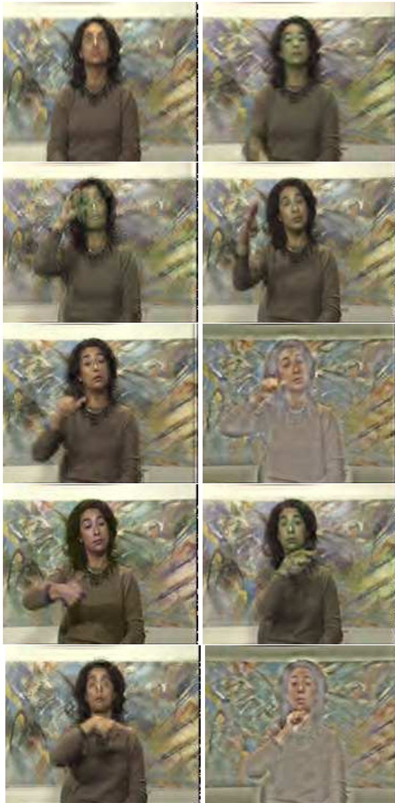
Figure 4.23: QCIF silent color video compressed at 200 kbits/s (30 frames/s). Transmission over UMTS Pedestrian channel at 0.01 ber. Using the SDC without channel coding.
