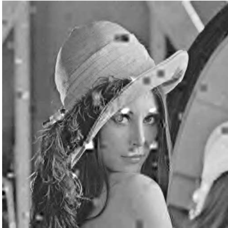
Figure 4.5: Lena image coded at 1.0 bpp. BSC channel at 0.01 ber. PSNR=24.99 dB.
