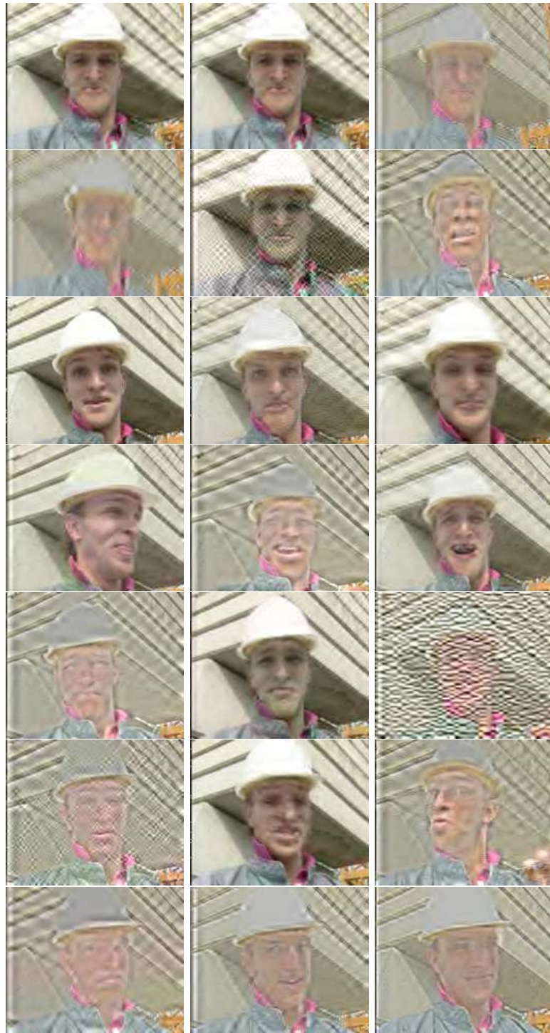
Figure 4.32: QCIF Foreman color video compressed at 200 Kbps (30 frames/s). Transmission over an Internet simulator suffering from 5 % packet loss. Using SDC. Y-PSNR: 20.50 dB; U-PSNR: 38.94 dB; V-PSNR: 40.62 dB.
