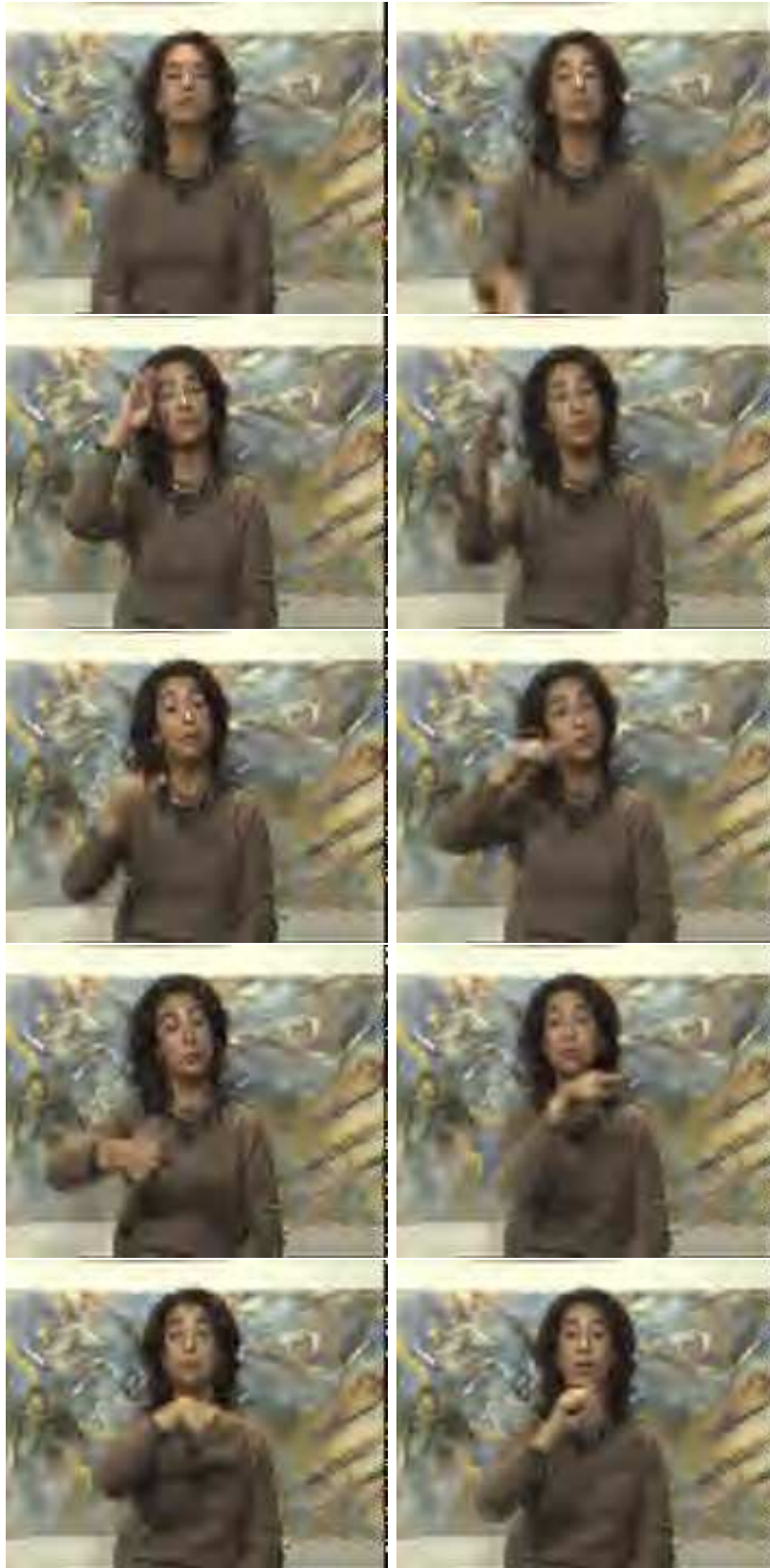
Figure 4.13: QCIF silent color video compressed to 200 kbits/s (30 frames/s). Transmission over Gaussian channel at 0.001 ber. Using the SDC+TC.
