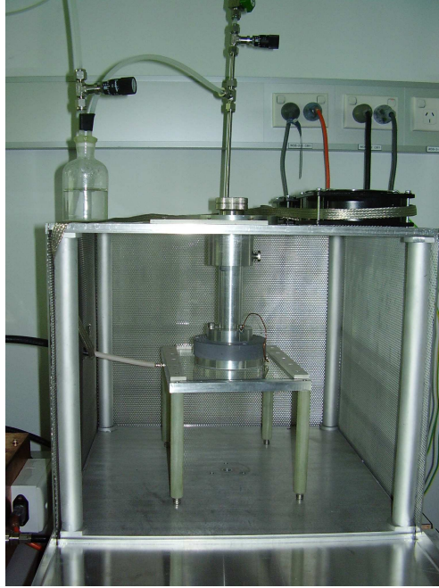
Figure 2.5: Optical set-up with transparent dielectric: Pyrex + fine copper mesh
