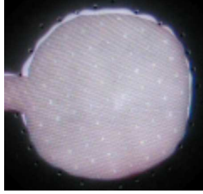
Figure 2.12: Axial view of plasma penetrating the “shower head” holes
