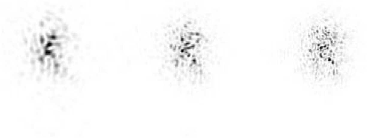
Figure 1. Speckle images with \frac{D}{r_0} = 10.33 for wavelength \lambda_0 , 17.77 for wavelength \lambda_1 and 26.62 for wavelength \lambda_2
