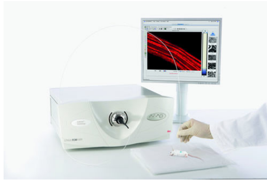
Figure 2.1: The Leica FCM1000 microscope (Cellvizio technology for small animal imaging distributed by Leica microsystems) used to image peripheral nerves of a mouse.
