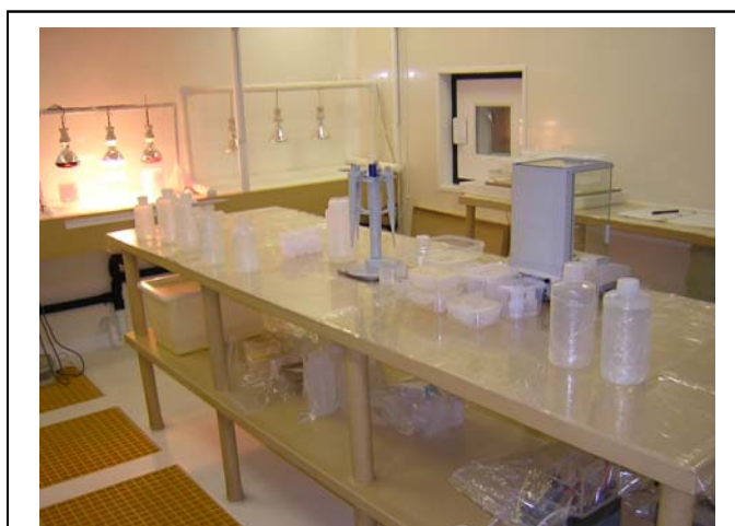
Fig. 5.2.1.1: Class 1000 Clean room with the class 100 laminar flow Teflon clean benches located inside the clean laboratory (containing infrared lamp) (CUT, Perth)
