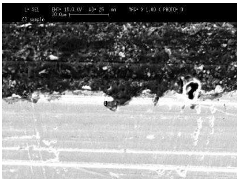
Figure 4.16: BSE micrograph of interface between opaque ceramic and palladium substrate.
