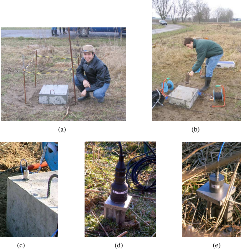
Figure E.3: Site of Lincint: (a) concrete foundation, (b) instrumented hammer, (c) accelerometer mounted on the foundation and (d, e) accelerometers in the free field.
