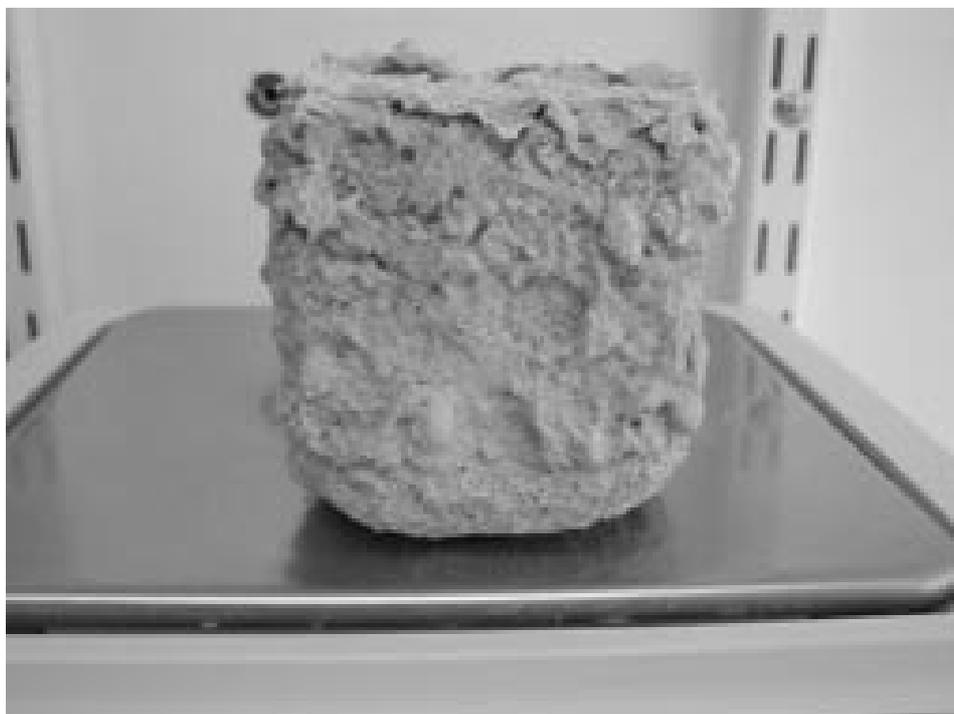
**Figure ART4-9a.** Picture of a  $7 \times 7 \times 7$  cm<sup>3</sup> non-isolated sample of FL after cycle 12.
