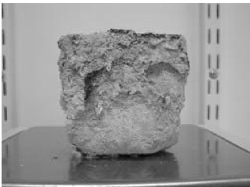
**Figure ART4-4b.** Picture of a  $7 \times 7 \times 7$  cm<sup>3</sup> sample of FL after 6 cycles of capillary imbibition & remobilisation.
