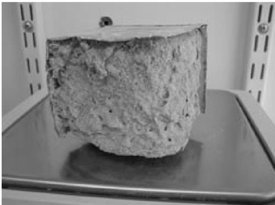
**Figure ART4-9b.** Picture of a  $7 \times 7 \times 7$  cm<sup>3</sup> sample of FL with 3 faces isolated after cycle 12.
