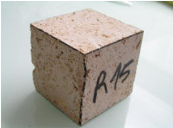
**Figure II-1.** Cube of 7cm side of the biotrititic cemented limestone RL ("roche franche").
