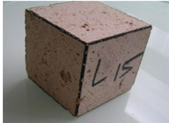
**Figure II-2.** Cube of 7cm side of the biotrititic cemented limestone LL ("liais").
