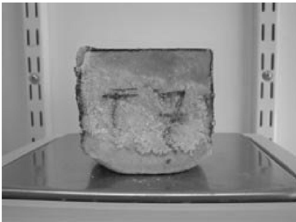
Figure ART4-2. 7x7x7 cm<sup>3</sup> sample with the four lower corners damaged (SF, capillary imbibition & remobilisation after 7 cycles).
