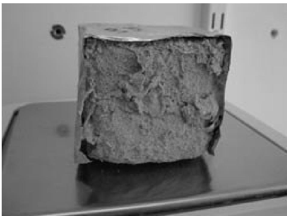
**Figure ART4-9c.** Picture of a  $7 \times 7 \times 7$  cm<sup>3</sup> sample of FL with 4 faces isolated after cycle 12.
