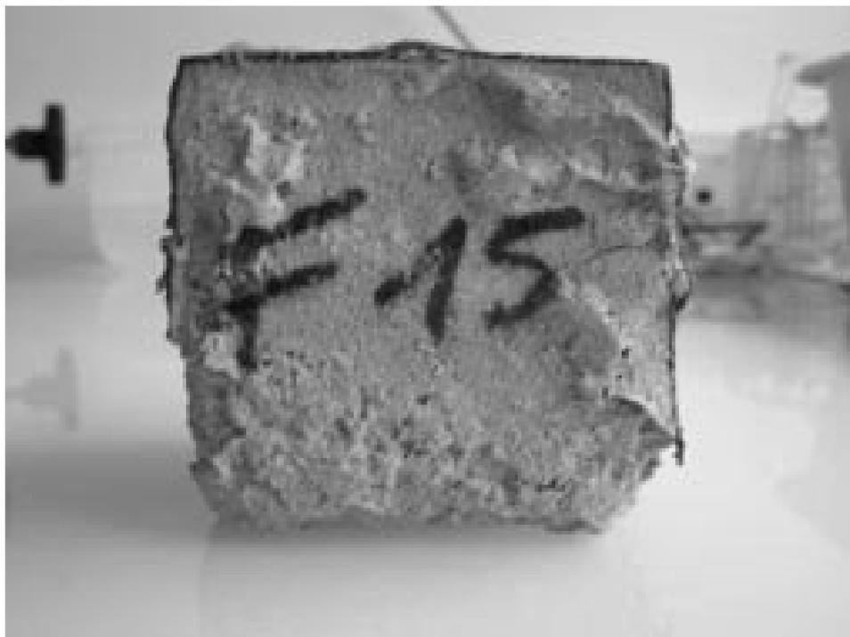
**Figure ART4-4a.** Picture of a  $7 \times 7 \times 7$  cm<sup>3</sup> sample of FL after 6 cycles of capillary imbibition.
