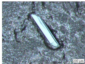
Single crystal of \text{Bi}_{0.45}\text{Dy}_{0.55}\text{FeO}_3 0.75 \times 0.15 \times 0.04 \text{ mm}^3 (optic)
