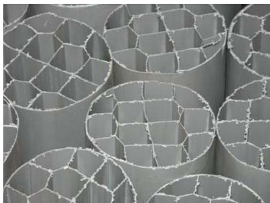
FIG. 2.4 – Support *Cloisonyle™* vierge
