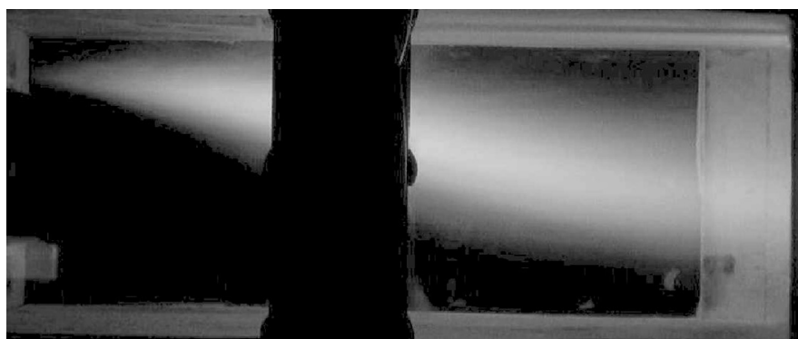
Figure 12. Direct emission of the flame in the case of \Phi(1) = 0.3 , \Phi(2) = 0.9 .
