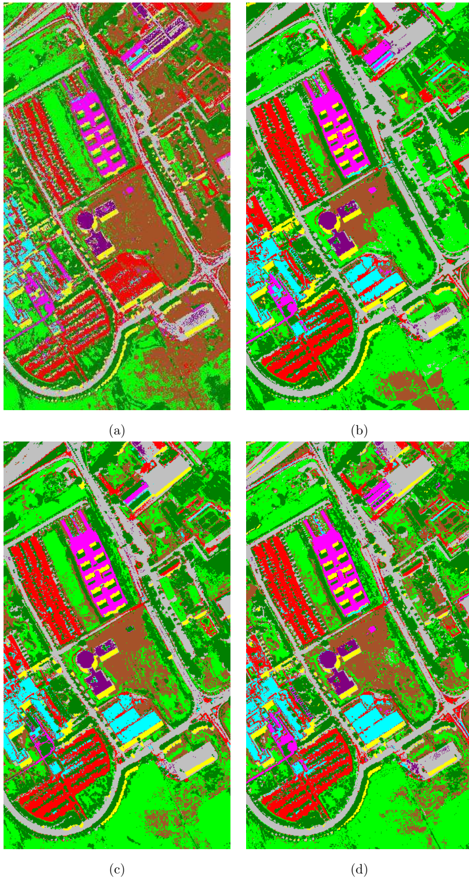
Figure 6.3: ROSIS University Area: Classification map obtained using SVM from: (a) original hyper-spectral data, (b) EMP, (c) 37 DBFE features, and (d) 13 NWFE features. Classification accuracies are reported in Tables 6.2, 6.3, 6.5, and 6.6.
