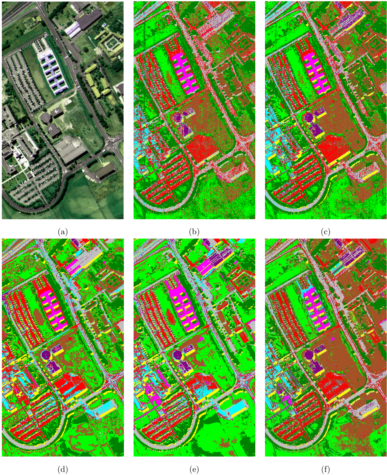
Figure 3.10: (a) False color original image of University Area, (b) Classification map using maximum likelihood, (c) Classification map using DBFE + ML, (d) Classification map using PCA+NN, (e) Classification map using ICA+NN, and (f) Classification map using SVM.
