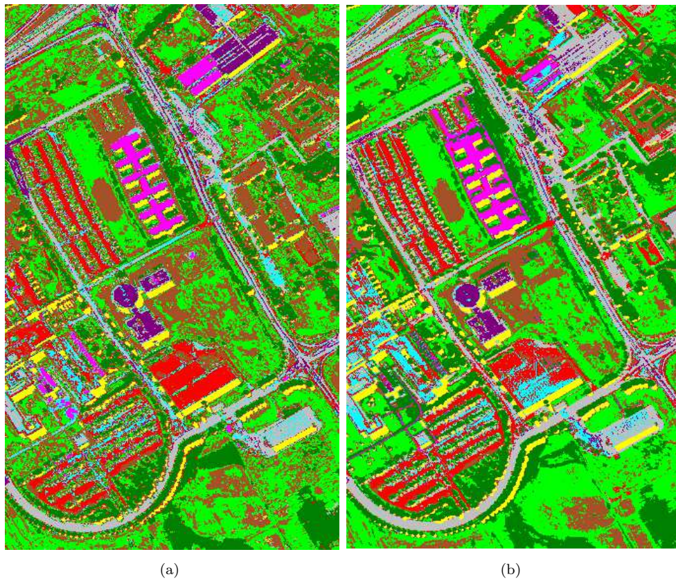
Figure 1.7: Classification map obtained (a) using a neural network and the first 8 KPCs and (b) from the first 11 KPCs with a linear SVM. Class descriptions: asphalt, meadow, gravel, tree, sheet metal, bare soil, bitumen, brick, shadow.
