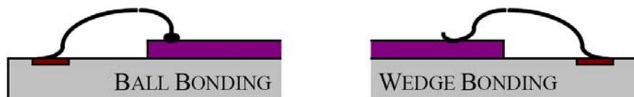
**Figure IV.35** Deux techniques de wire bonding
