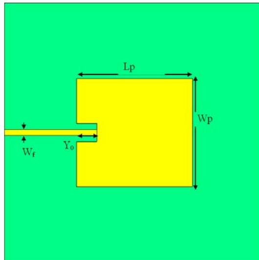
Figure III.33 Antenne patch
