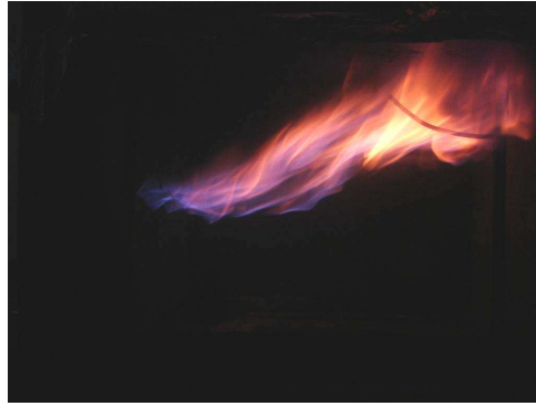
Fig. 3.31: View from the side of the flame for a fuel flow rate of 0.71 \text{ g/s} [ \dot{H} = 33 \text{ kW} ] and a vent width of 0.05 \text{ m} = 0.125 W
