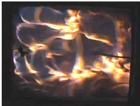
Fig. 3.6: View of the flame from underneath taken through the window in the floor of the compartment: line burner, large soffit, 0.63 \frac{s}{s} fuel flow rate ( \dot{H} = 29 kW), unrestricted vent
