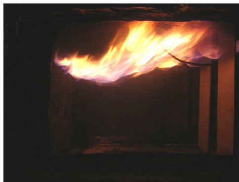
Fig. 3.30: View from the side of the flame for a fuel flow rate of 0.71 s/s [ \dot{H} = 33 kW] and a vent width of 0.1 m = 0.25 W
