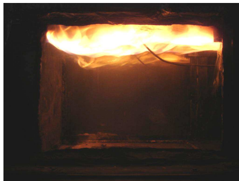
Fig. 3.28: View from the side of the flame for a fuel flow rate of 0.71 \text{ g/s} [ \dot{H} = 33 \text{ kW} ] and a fully open vent
