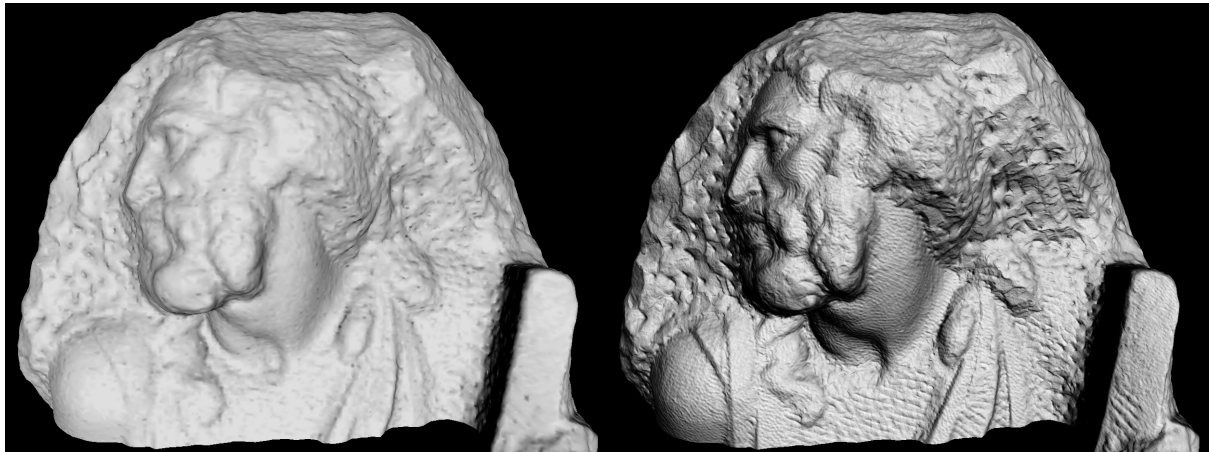
Figure 6.7: Upper part of the St Matthew model with our method rendered at 165 FPS, without (left) and with (right) the normal maps. The maps are recreated directly from the point cloud, providing a convincing appearance, while using less than 80k triangles (left image). Most of the “appearance” information carried by the original point cloud is directly stored through these normal textures on the GPU memory (185 MB) and used for the per-pixel lighting.
