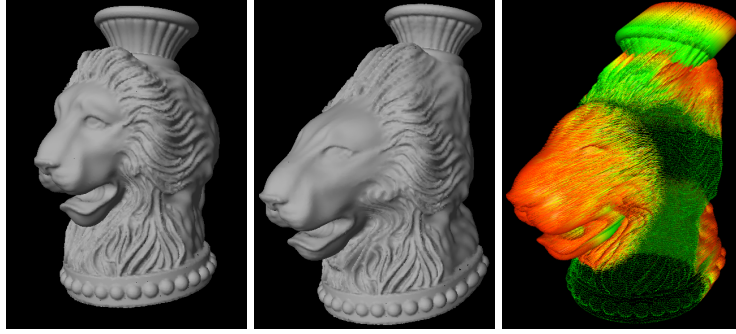
Figure 4.6: Left: Initial in-core geometry obtained by out-of-core VS-Tree clustering. Middle: Deformed in-core geometry after an interactive FFD session. Right: Discrete displacement field generated by linking the initial (green extremum) and the final (red extremum) position of each sample point. This displacement field performs a sampling of the continuous space deformation function at the scale at which it has been edited.
