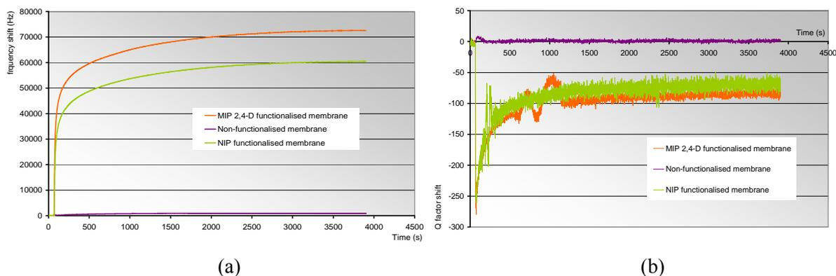
**Figure 2.33:** Real-time (a) resonant frequency and (b) quality factor variations during the polymerization phase of the MIP and NIP, respectively, compared to the output signal of a non-functionalized membrane
