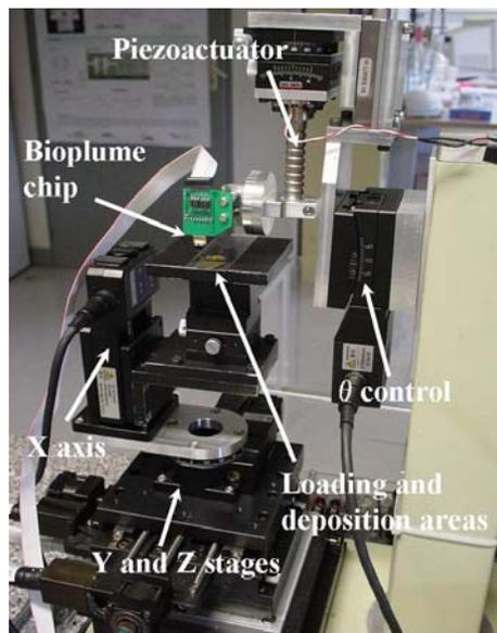
**Figure 2.9:** Picture of the four-degree-of-freedom depositing spotter including the cantilever array<sup>88</sup>.
