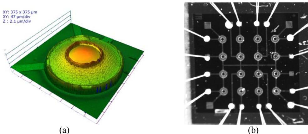
**Figure 2.25:** **a)** 3D static profile (obtained by optical interferometry) of a single piezoelectric membrane; **b)** Optical microscope photograph of 5x5 mm<sup>2</sup> chip of 4x4 membranes matrix with wire connections
