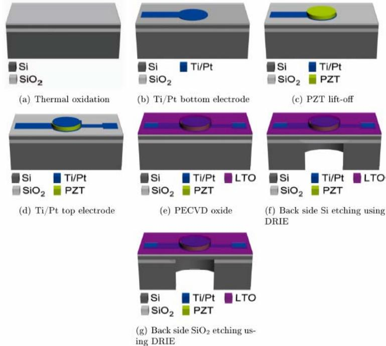
**Figure 2.14:** Fabrication steps of piezoelectric circular micromembranes
