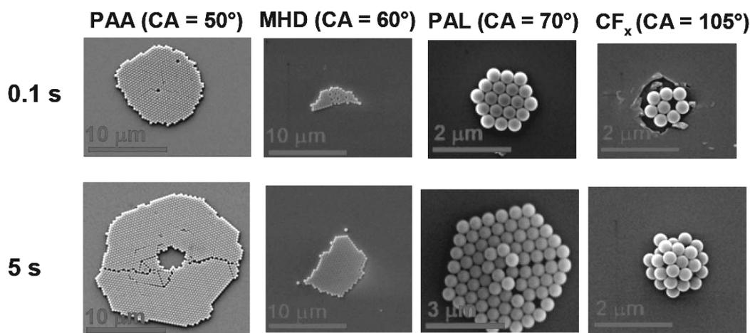
**Figure 2.12:** SEM pictures of the microspots of PS nanoparticles on the different substrates (polyacrylic acid (PAA), polyallylamine (PAL), fluorcarbon (CF<sub>x</sub>) and mercaptohexadecanoic acid (MHD)) for the minimum (0.1 s) and the maximum (5 s) contact time<sup>88</sup>.
