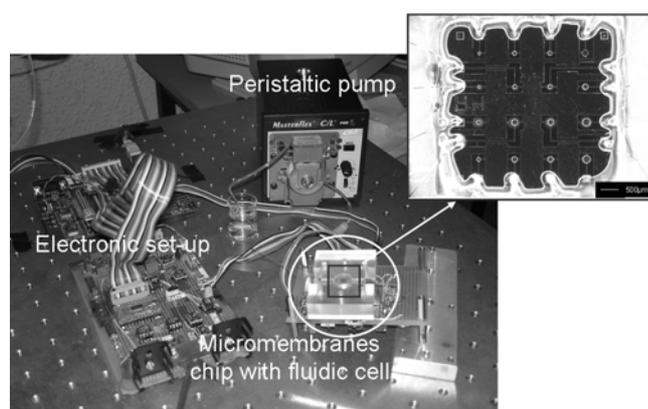
**Figure 2.28:** Photograph of the global system with the electronic set-up, the liquid injection pump and the fluidic cell including the membranes chip. The inset shows a top view of a chip with the fabricated micromembranes, the wire-bondings and the silicon sealant.
