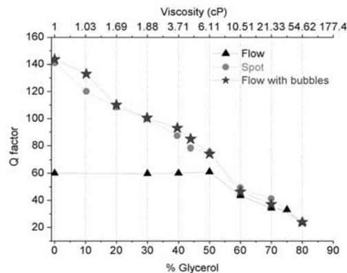
**Figure 2.20:** In-spot, in-flow and in-flow with air bubbles measured quality factors of a piezoelectric membrane ( $R_2 = 100\mu\text{m}$ ,  $R_1/R_2 = 0.5$ ) versus glycerol proportion in aqueous solutions.
