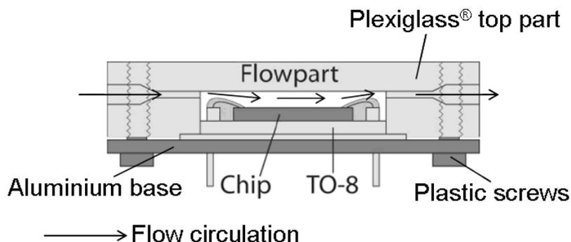
**Figure 2.18:** Schematics of the flow-through cell (not to scale). The top part is fabricated in Plexiglas™, the base in aluminium and the TO8 package of the piezoelectric membranes matrix is held together with the fluidic cell parts with four plastic screws.
