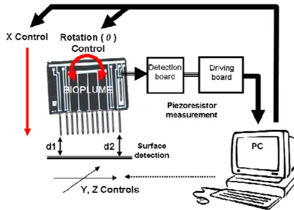
**Figure 2.8:** Diagram of the closed-loop Bioplume spotter<sup>88</sup>.
