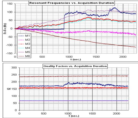
**Figure 2.22:** Resonant frequencies and corresponding quality factors stability of 6 piezoelectric membranes measured by means of the proposed electronics (except M3 and M4 that are identical, all the other devices have different piezoelectric patch diameters thus explaining the different behavior in time)
