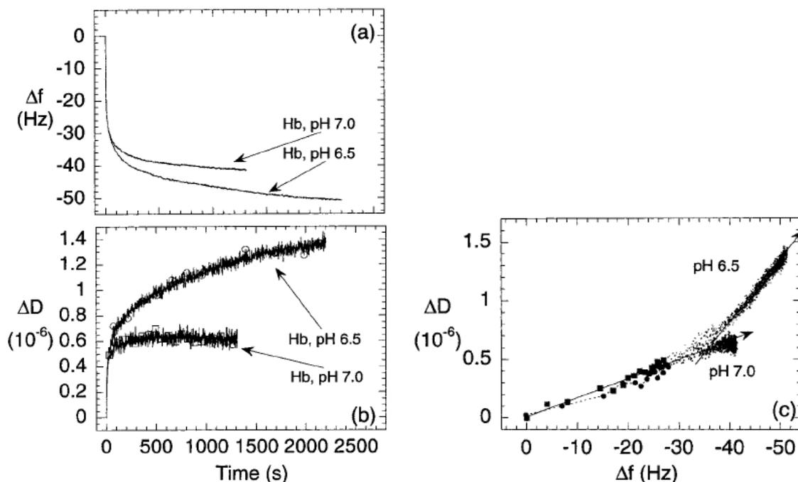
**Figure 1.9:** (a, b)  $\Delta f$  vs  $t$  and  $\Delta D$  vs  $t$  for the adsorption of Hb on the hydrophobic surface at pH 6.5 and 7.0. The influence of pH on the Hb adsorption kinetics is also illustrated by the  $D$ - $f$  plot (c). The simple linear behavior at pH7.0 is replaced by a two-phase behavior at pH6.5, where also the total mass uptake and final dissipation shift are larger. (●) pH7.0 and (■) pH6.5.
