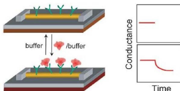
**Figure 1.10:** Schematic of a Si nanowire-based FET device configured as a sensor with antibody receptors (*Y-shaped*), where binding of a protein with net positive charge yields a decrease in the conductance (upon Patolsky and Lieber<sup>228</sup>)
