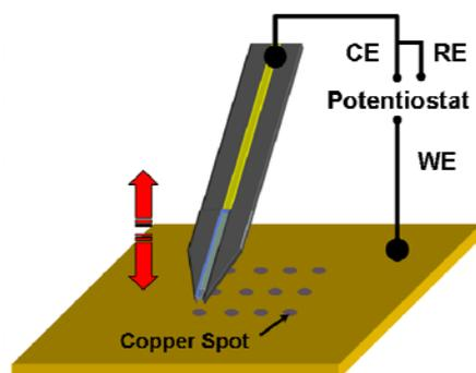
**Figure 2.13:** Schematic of the experimental setup<sup>88</sup>.
