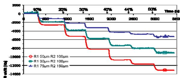
**Figure 2.24:** Real time measurement of resonant frequency evolution of three piezoelectric membranes for the injection of different water/Glycerol mixtures (0, 10, 20, 30, 40, 44 and 50% of glycerol diluted in water)
