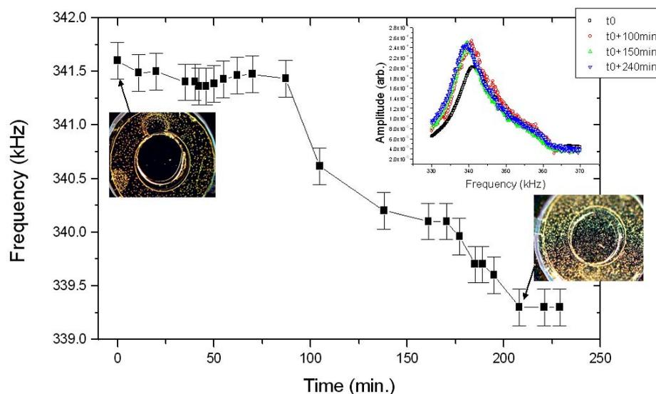
**Figure 2.26:** Evolution of the (0,1) resonant frequency of the piezoelectric membrane vs. time during the injection of a colloidal solution (at pH 5.3) into the reaction chamber of the flow-through system. The two optical microscope photographs show the piezoelectric membrane before and after adsorption of gold colloids on its surface. Error bars represent the standard deviation of the measured resonant frequency during 5 experiments.
