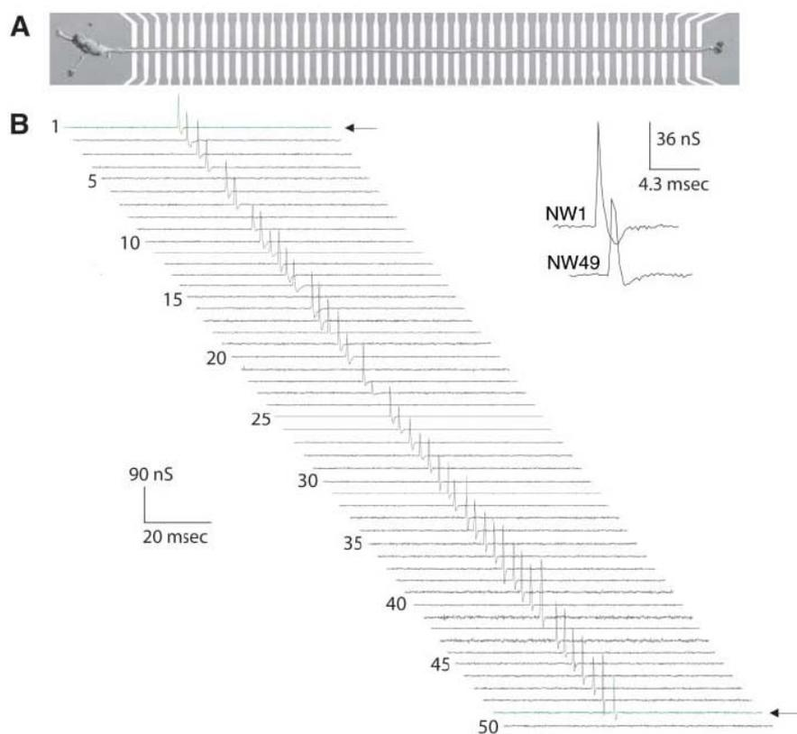
**Figure 1.12:** Highly integrated NW-neuron devices. (A) Optical image of aligned axon crossing an array of 50 NW devices with a 10-mm interdevice spacing. (B) Electrical data from the 50-device array shown above. The yield of functional devices is 86%. The peak latency from NW1 (*top arrow*) to NW49 (*bottom arrow*) was 1060 ms (courtesy from Ref.<sup>234</sup>, © 2006 Science)
