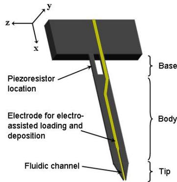
**Figure 2.1:** 3D schematic of the Bioplume cantilever showing the working coordinate system used in the following calculations.
