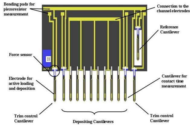
**Figure 2.3:** Schematic of the Bioplume array.
