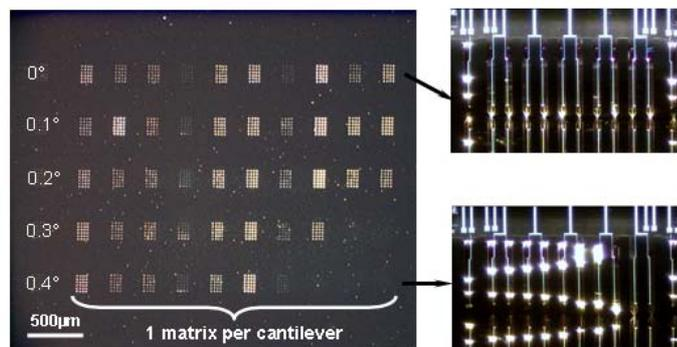
**Figure 2.10:** *Left:* Photograph of water-glycerol droplets' matrices realized by increasing the misalignment of the array. *Right:* Optical photographs of the array while depositing for 2 different tilt angles (Top:  $0^\circ$ . Bottom:  $0.4^\circ$ )<sup>88</sup>
