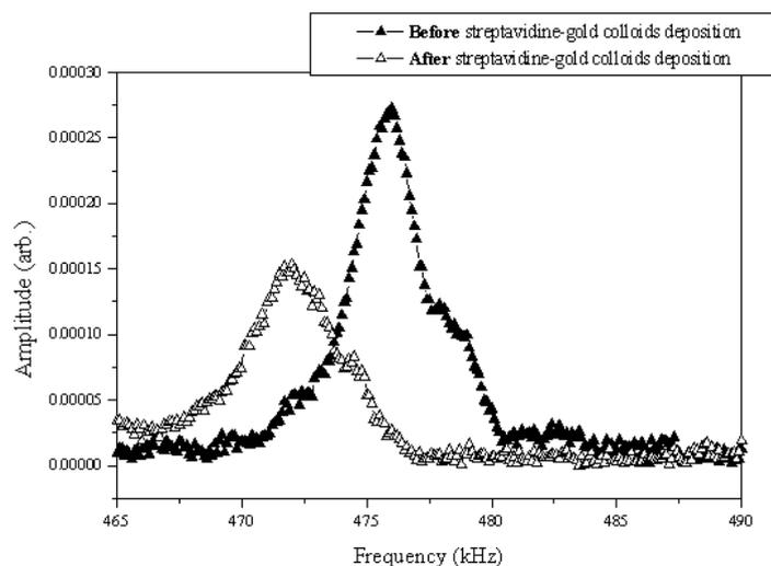
**Figure 2.27:** (0,0) resonant frequencies measured before and after the deposition of streptavidin-conjugated gold colloids on the surface of a piezoelectric membrane where biotinylated DNA oligonucleotides were previously hybridized with complementary oligonucleotides sequences
