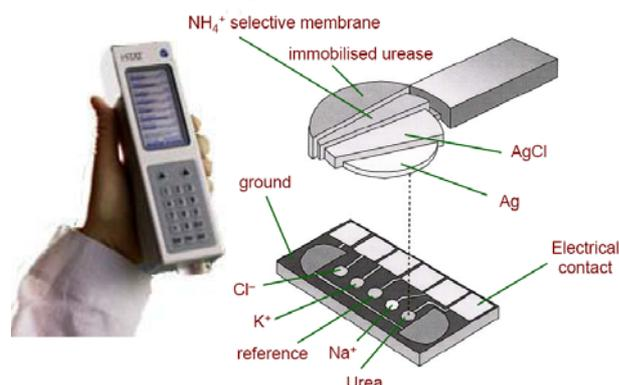
**Figure 1.4:** The i-STAT multisensor for monitoring various blood electrolytes, gases and metabolites<sup>18</sup>
