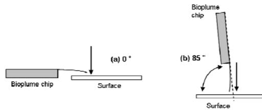
**Figure 2.7:** Lateral (a), and axial (b) bending conditions. The axial condition corresponds to the deposition configuration<sup>88</sup>.
