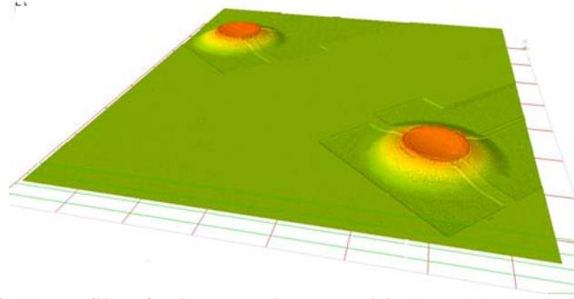
**Figure 2.15:** Typical 3D profile of micromembranes with  $R_1 = 75 \mu\text{m}$  and  $R_2 = 200 \mu\text{m}$  obtained using a Fogale<sup>©</sup> interferometer
