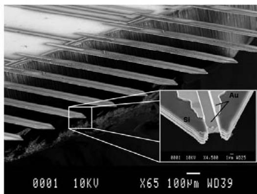
**Figure 2.5:** SEM picture of a cantilever array with SEM close-up view of the silicon tip showing the electrode inside the fluidic channel.
