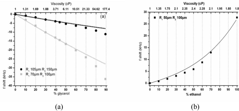
**Figure 2.19:** (a) Resonant frequencies shift as a function of glycerol content for two piezoelectric membrane designs ; (b) Resonant frequency shift as a function of ethanol content for a piezoelectric membrane ( $R_2 = 100\mu\text{m}$ ,  $R_1/R_2 = 0.5$ ). Symbols stand for experimental values while line stands for theoretical data.
