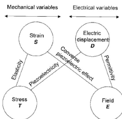
**Figure 1.7:** Relationship between mechanical and electrical variables. The direct piezoelectric effect is the production of electric displacement by applying a mechanical stress. The converse piezoelectric effect results in a strain in the crystal when an electrical field is applied. The relation between stress and strain is determined by the elasticity of the solid<sup>177</sup> (courtesy of *Angewandte Chemie* editorial board)
