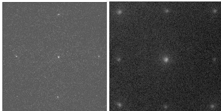
Figure 3.30. LEED patterns of the (001) STO single crystal substrate (left) showing no reconstructed surface and of the LSMO film deposited on it (right) showing itself no reconstruction.
