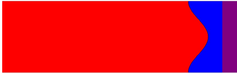
FIG. 2.17 – Initial geometry, a shock wave is propagating in the water from right to left. A sinus shape interface between air at left and water at right.
