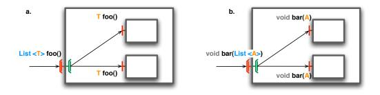
Figure 4.4: Component systems using multicast interfaces
