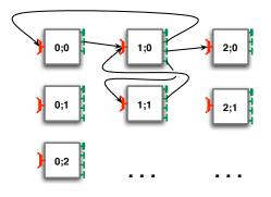
**Figure 6.9:** Jacobi computation: borders exchanges through collection and gathercast interfaces (communications are represented only for component (1;0))
