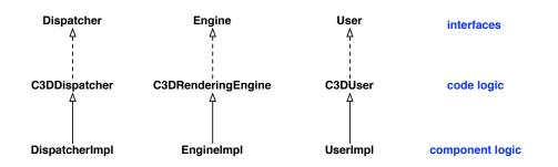
Figure 6.1: C3D component classes and interfaces
