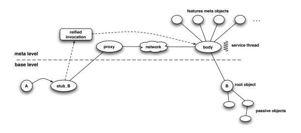
Figure 2.13: Meta-object architecture
