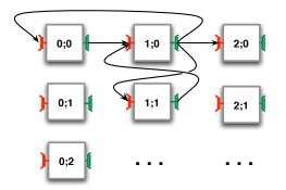
**Figure 6.8:** Jacobi computation: borders exchanges through multicast and gathercast interfaces (communications are represented only for component (1;0))
