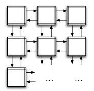
**Figure 6.7:** Jacobi computation: matrix elements exchange border data with their neighbors during computation
