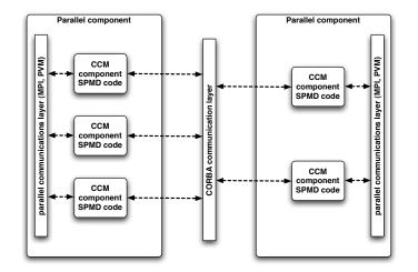
Figure 2.11: Coupling of parallel components with GridCCM
