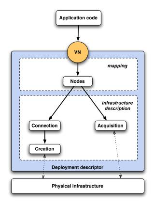
Figure 2.15: Descriptor-based deployment
