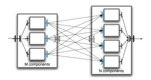
**Figure 4.12:** An optimized implementation for the MxN problem based on local multicast and gathercast interfaces
