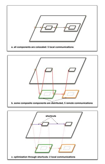
Figure 5.6: Using short cuts for minimizing remote communications
