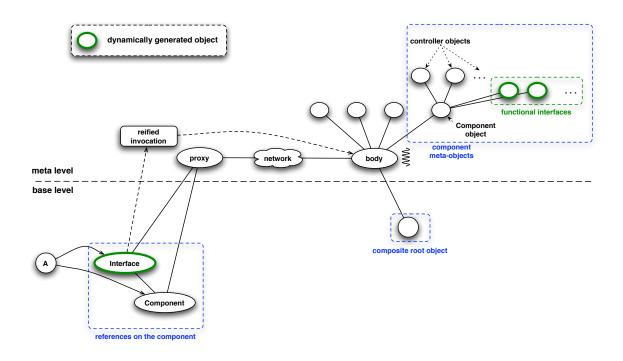
Figure 5.2: ProActive Meta-Object architecture for composite components
