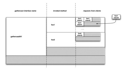
Figure 5.9: Data structure for the buffering of requests in gathercast interfaces
