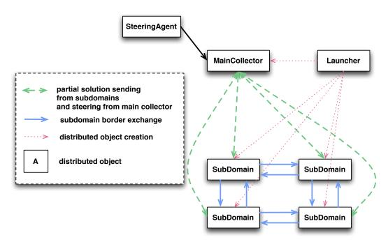
Figure 6.2: Original Jem3D architecture following an object-oriented design
