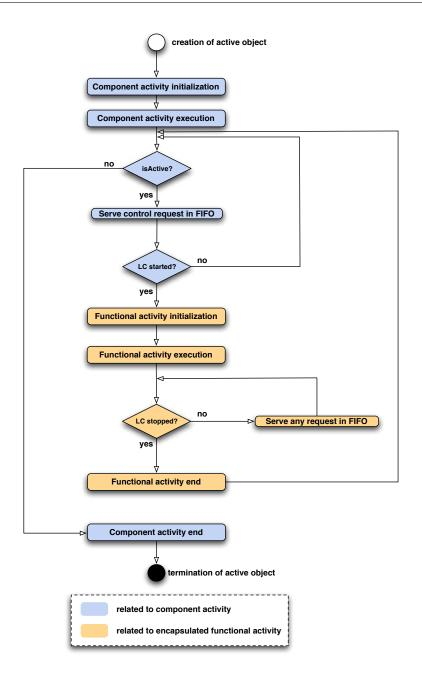
Figure 5.3: Default encapsulation of functional activity inside component activity
