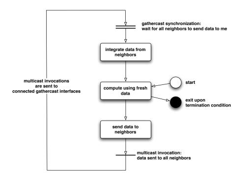
Figure 4.9: A typical algorithm for SPMD components
