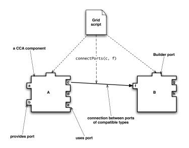
Figure 2.6: An assembly of CCA components
