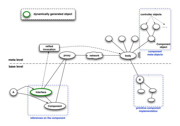
Figure 5.1: ProActive Meta-Object architecture for primitive components
