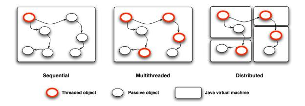
Figure 2.12: Seamless sequential to multithreaded to distributed objects
