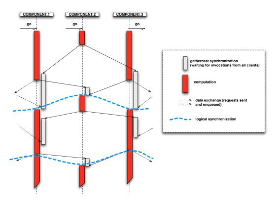
Figure 4.10: Synchronization between components in a SPMD computation
