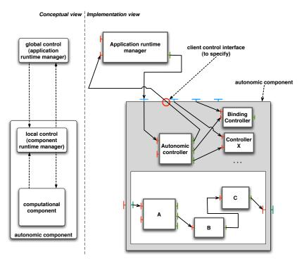
Figure 7.4: Autonomic components in ProActive / GCM
