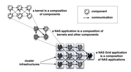
Figure 3.1: A conceptual view of the hierarchical structuration of a NAS Grid benchmark
