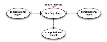
Figure 2.9: ODP compound binding
