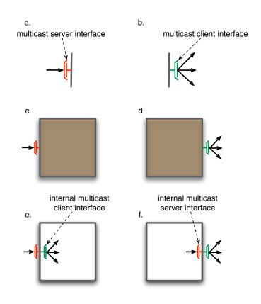
Figure 4.3: Multicast interfaces for primitive and composite components
