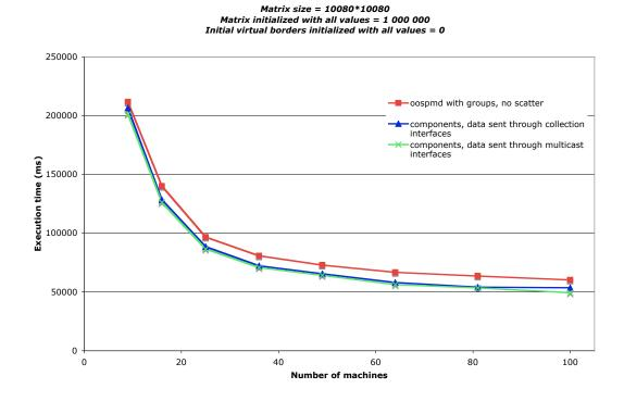
**Figure 6.10:** Jacobi computation benchmarks: comparing ProActive OOSPMD, components using multicast and components using collection interfaces for sending data
