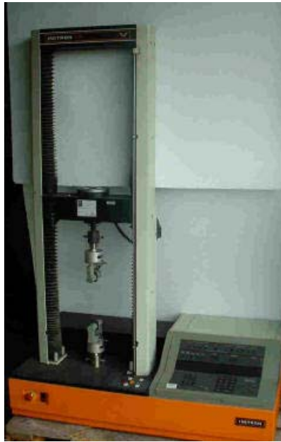
Figure II-12 : Machine de traction Instron 4301.
