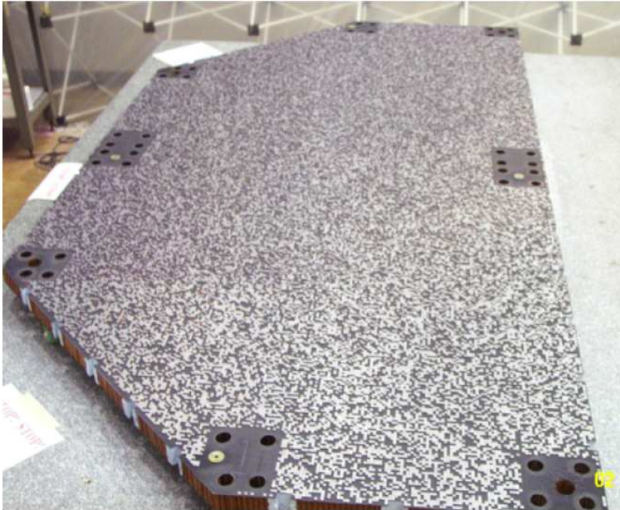
Figure 2.3: Picture of the BAT coded aperture mask before Swift launch.
