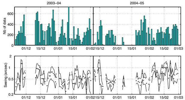
**Fig. 4.** Top: number of seeing data per day. Bottom: points are daily median seeing values and intervals containing 50% of values is delimited by lines. Data collected during the last two summer campaigns. Seeing axis is logarithmic
