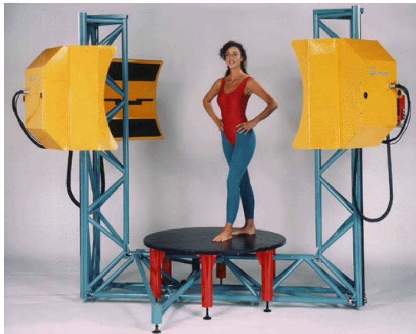
Figure 1.6. Full human body scanner. Courtesy of Cyberware.
