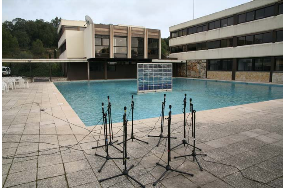
Figure 6.13 Microphone setup used to record the fountain example. In this case the microphones are placed at the center of the action.
