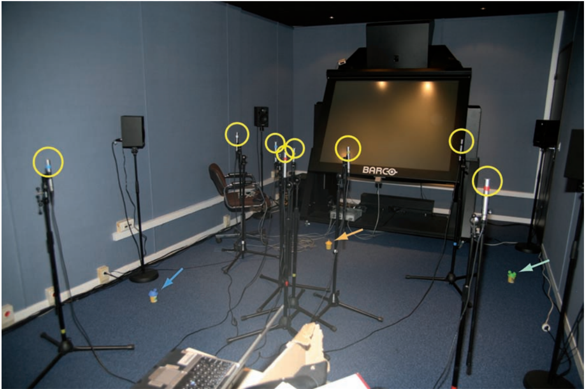
Figure 6.6 Indoor validation setup using 8 microphones. The 3 markers (see blue, yellow, green arrows) on the ground correspond to the location of the recorded speech signals.
