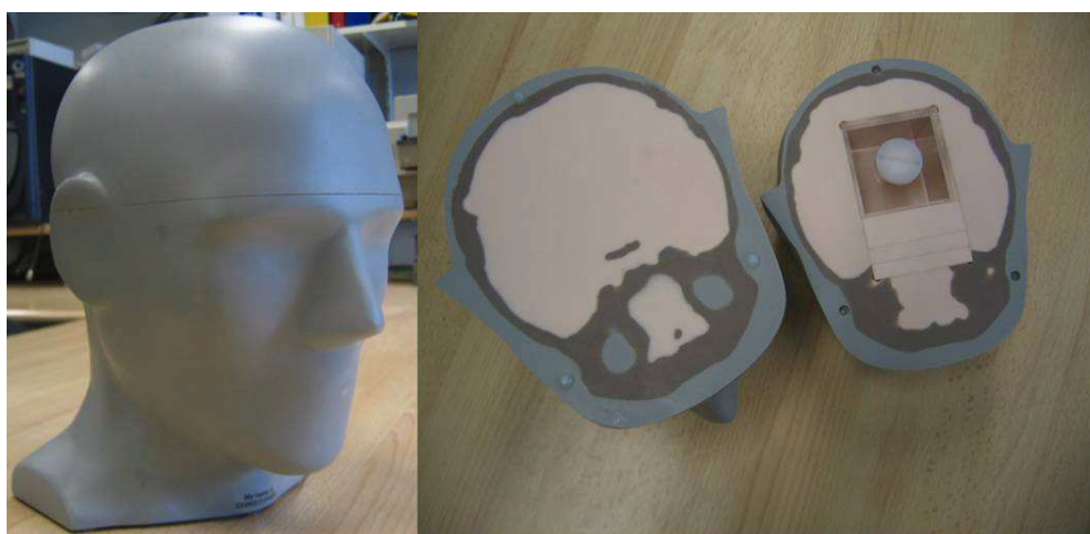
Figure 1. An anthropomorphic head phantom. Overview on the left side and opened phantom on the right. A cassette and three spacers are visible.
