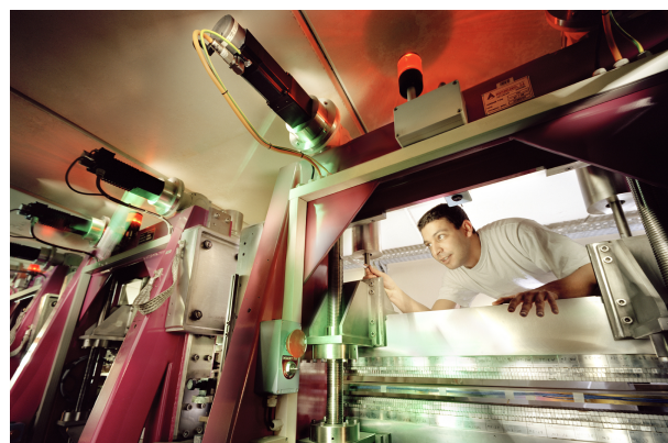
Figure 1.10 : Photo of an Undulator. Undulators are the brightest sources of photon beams in synchrotron radiation facilities. ©P.Ginter/ESRF
