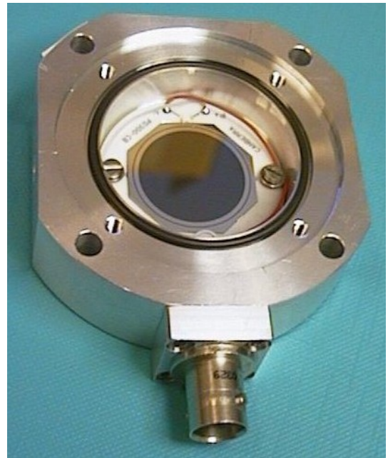
Figure 1.17 : A Photodiode used to monitor the beam intensity in its protecting case.
