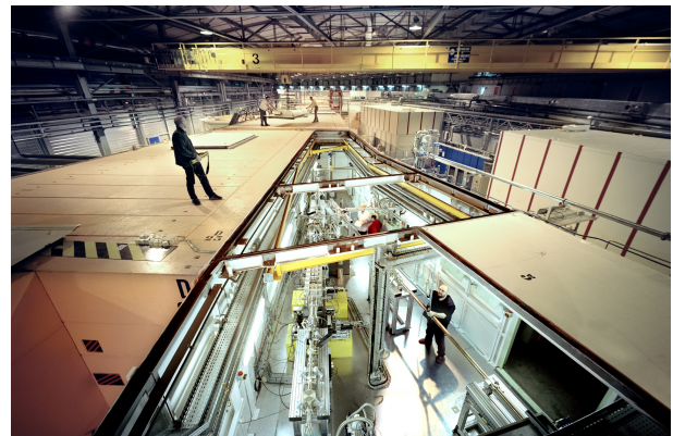
Figure 1.12 : A beamline seen from the top. The storage beam is hidden behind the concrete blocks on the left side of the picture. Photons enter the beamline at the top of the photo. ©P.Ginter/ESRF
