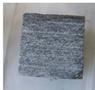
Figure 2.8 : composite KNO<sub>3</sub>/NaNO<sub>3</sub> + 10%<sub>m</sub> de GNE.
