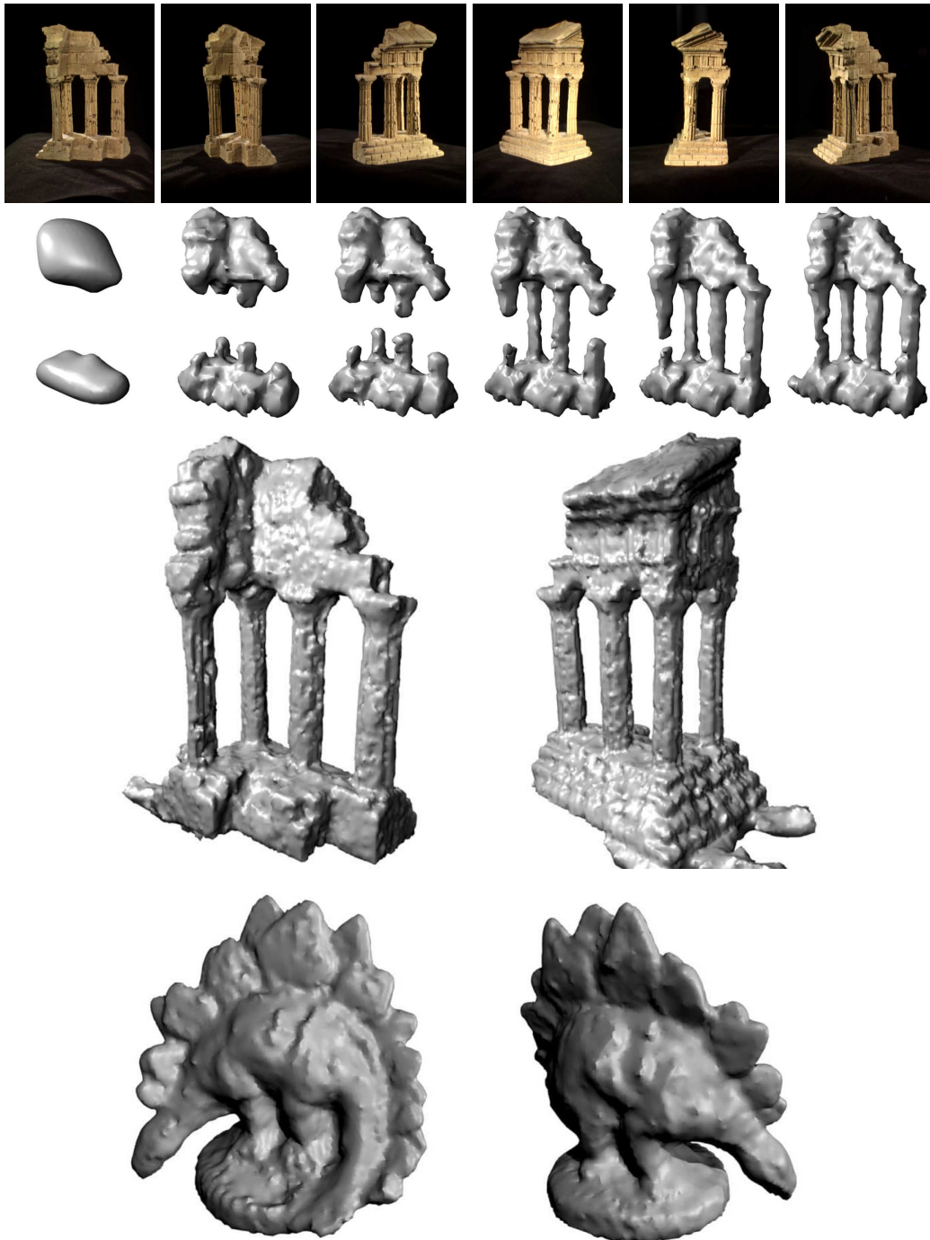
Figure 5.10: First row: some of the input images of the temple dataset. Second row: surface evolution for the temple sparse ring dataset. Third row: final reconstruction for the temple sparse ring dataset. Forth row: final reconstruction for the dino sparse ring dataset.
