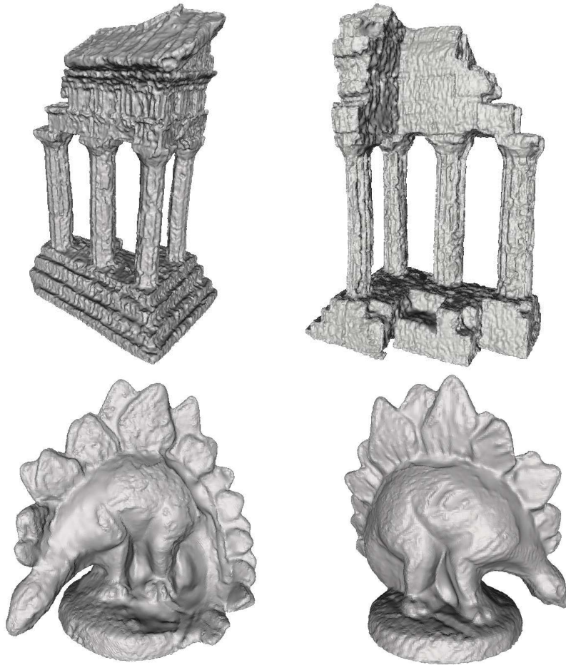
Figure 5.12: Reconstruction obtained for the temple ring and dino ring datasets, while estimating the specular component and the background.
