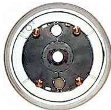
HERA B=4.7 T Bore: 75 mm
