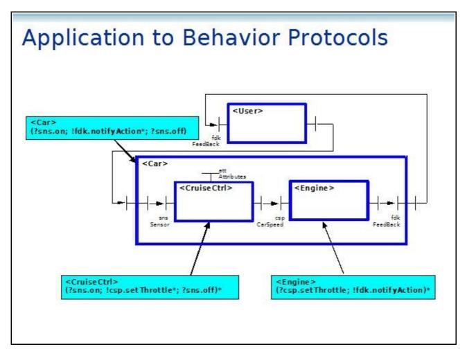
I'm going to illustrate how the formalism adapter models specifications and help to build the contract between the Car, the CruiseCtrl and the Engine, with the behavior protocols formalism.
