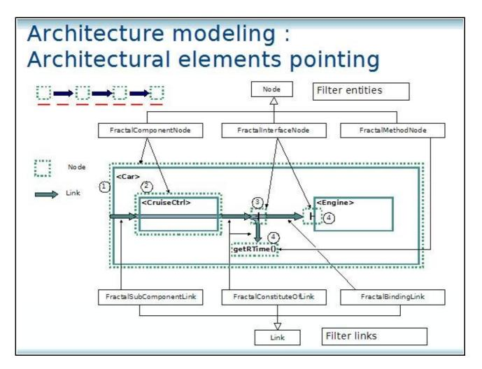
This is an example of two paths : both starting at the Car component and for one finishing on an interface of Engine component, for the other on the method getRTime of an interface of the CruiseCtrl.
