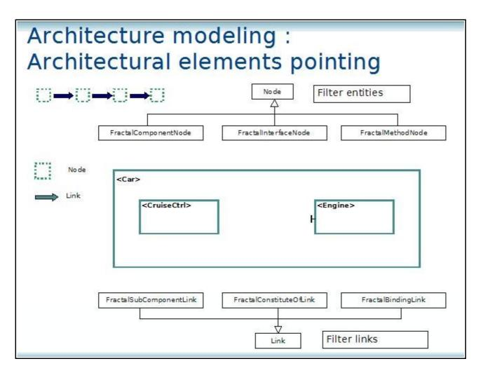
I give here an example of specialization of the Node and the Link for the Fractal component model :
