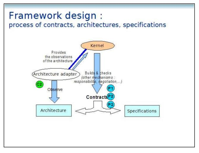
so in order to build contracts that apply to a given architecture, the kernel which is generic, uses an "architecture adapter" that observes the architecture and describes it in the generic terms defined by the kernel.
