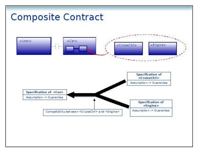
In this case the specification expression of the composite component (Car) is mechanically deduced from the ones of the subcomponents (Engine and CruiseCtrl), and is valid as long as the agreement of the contract between the subcomponents holds.
