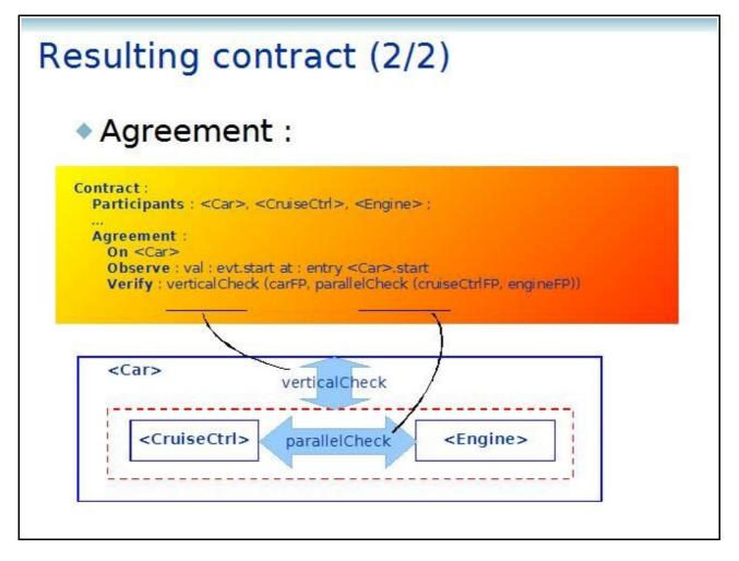
So the expression of the agreement is composed of an horizontal modelcheck of components at the same level of composition, and a vertical modelcheck between the group of subcomponents and the composite.
