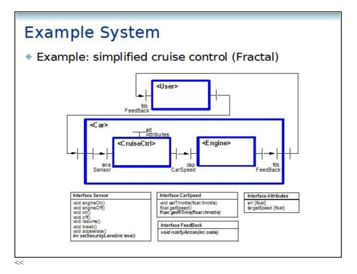
to illustrate the following of the presentation, I will consider a very basic components system. Components are the blue rectangles, they are bound through interfaces drawn as horizontal "T". Server interfaces are on the left of the component client ones are on their right side. I take a hierarchical component model, such as the "Fractal Component Model" (developed at France Telecom R&D).
