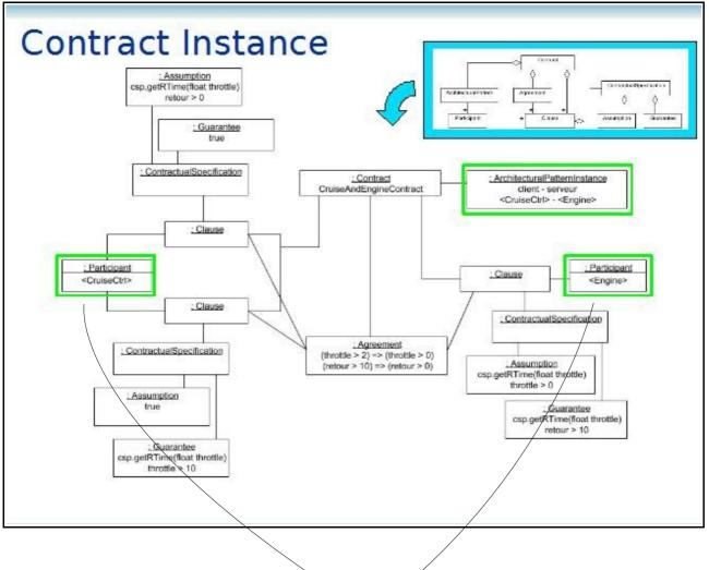
the architectural pattern is used to distinguish the participants of the contract, then the relation between the participants, pointed by the pattern, is used to retrieve the specifications that constrain what is exchanged on it.
