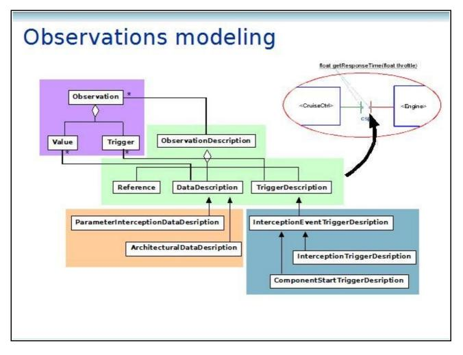
So the observation mechanism specialized by the architecture adapter then provides, for a given ObservationDescription, an Observation containing the value of the data, and the concrete values concerning the triggering of the observation.
