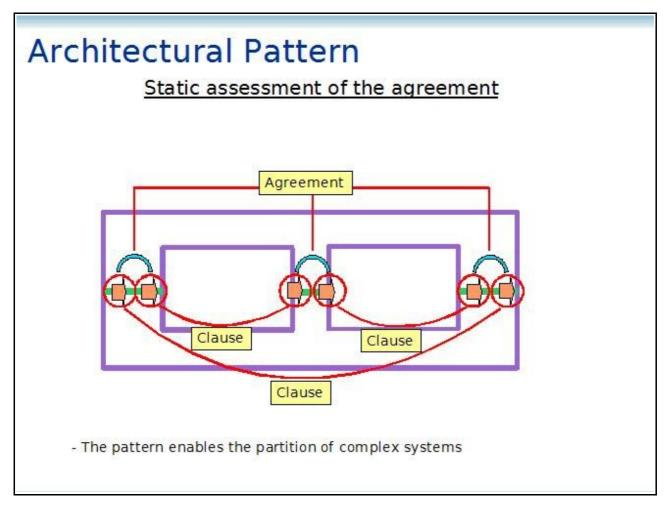
The agreement of the contract reifies the compatibility of the clauses : that is : on each link, each emitted message by a component (according to its clause) corresponds to a message awaited by one other component (according to its clause).
