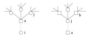
Figure 1.4: Parts of the factor graph used to compute  $\psi_{s_i}^{a \to i}$  and  $\chi_{s_i}^{j \to a}$ .
