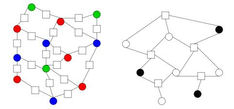
Figure 1.1: Example of a factor graph representation for the coloring (left) and the exact cover (right) problems. The function nodes (squares) in the graph coloring are satisfied if and only if their two neighbours (circles) are in different states (take different colors). The function nodes (squares) in the exact cover problem are satisfied if exactly one variable (circle) around them takes values 1 (full) and the others 0 (empty).
