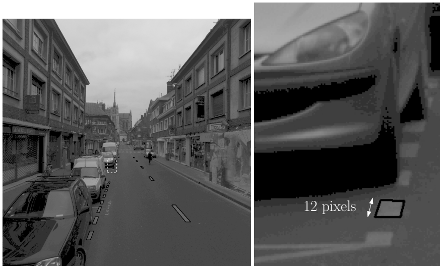
(a) Images resolution: 4096 \times 4096 , the reconstruction is efficient until distance of 30 m from camera.
