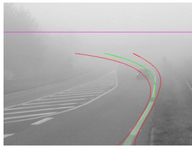
Figure 2.16: According to [Ieng et al. , 2004]: Curve fitting result under foggy conditions (green curve) and uncertainty curves (red curves).
