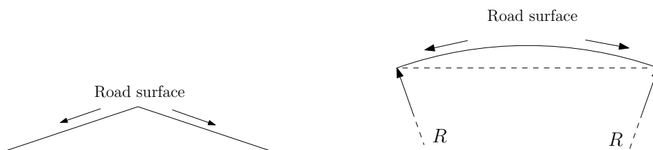
Figure 2.4: Two kinds of road section: sloped and curve surfaces are applied to guide raining water to the borders.
