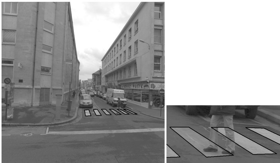
Figure 6.3: Extraction under partial occlusion of strip's sides.
