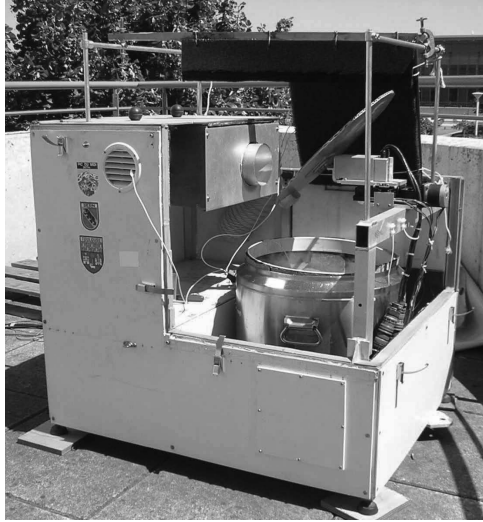
Fig. 1. The MobRa instrument for the measurement of middle atmospheric H 2 O on the terrace of the Laboratoire d'Aérodologie, Toulouse, France.
